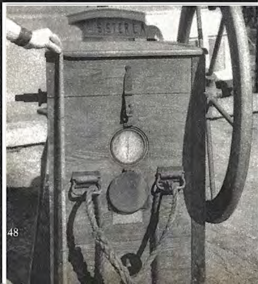
The diver above is ready for a plunge to the ocean bottom where gold or death awaits him. Pressure pump below supplies air—60 pounds at 100 feet.
