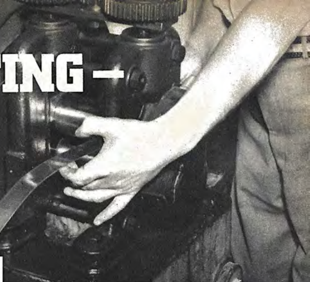
Machinery is used only at the start of the goldbeating process. The gold is flattened into ribbon form between rollers of a press, as shown in above photo.
