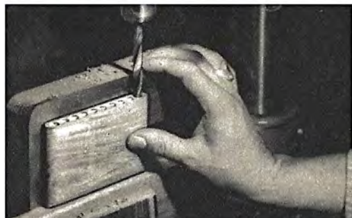
The cigarette case completed and ready for use is shown in the top photograph. Above is shown the case being drilled. Use a drill size only slightly larger than the cigarette diameter.
