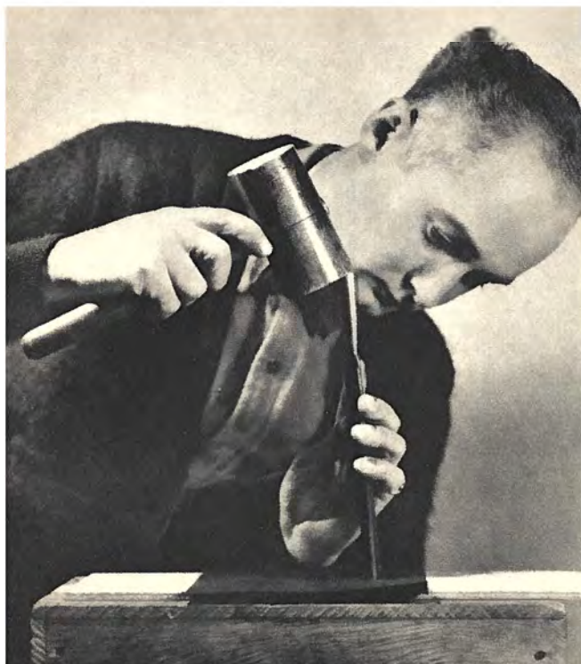
A concave chisel can be used for cutting masks having round-cornered openings.
