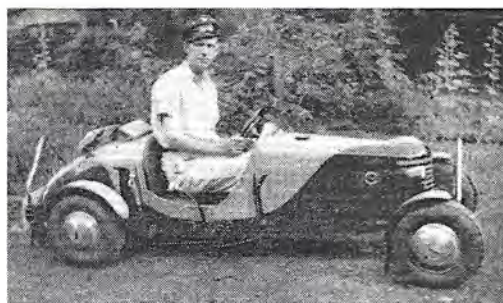
Powered by a 3½ horsepower motor, this trim looking midget racer carries builder William Walker at speeds up to 45 m.p.h.
