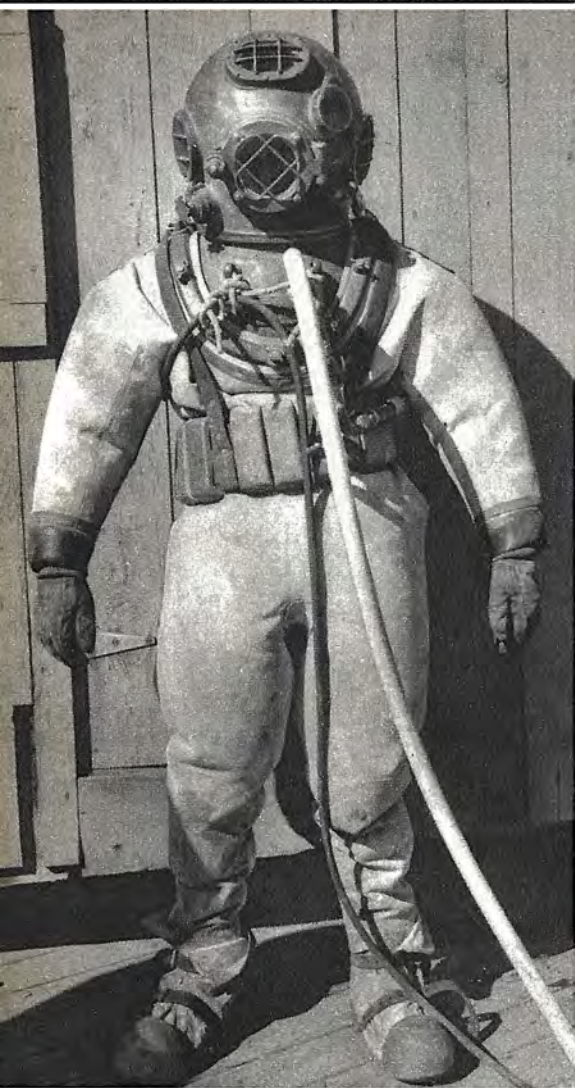
The diver above is ready for a plunge to the ocean bottom where gold or death awaits him. Pressure pump below supplies air—60 pounds at 100 feet.
