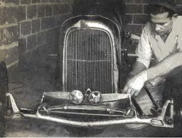
Every driver has his own ideas about how a midget should be built. Jack Yisitis (above) swears by his tubular axle.
