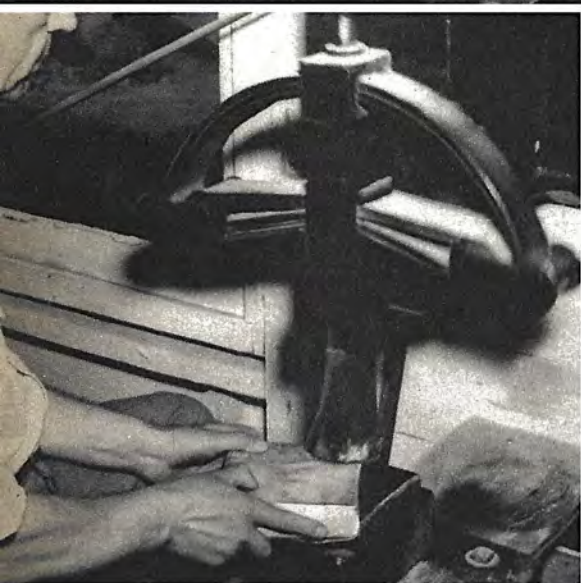
Goldbeater's skin, used to cover the gold leaf during the beating process, must be conditioned by subjection to trip hammer blows for 40 minutes before use (above).
