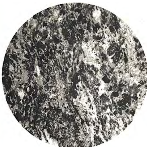
A professional slide of chlorite schist prepared as a thin section for study by transmitted light. Such a slide reveals the details of rock structure.
