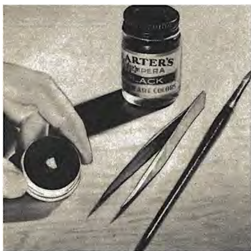
A circular pill box with sunstone specimen mounted on a cork pyramid in the center, for low power examination with strong reflected light. The box interior is painted black.
