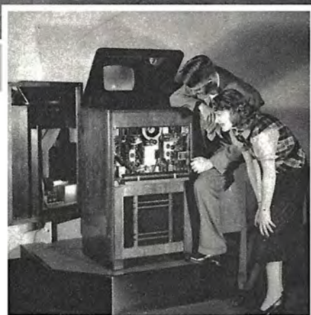
Above—The equipment in this receiver-monitor is enclosed in glass for the benefit of visitors on the television tour. Below—A simplified diagram of the television demonstration equipment.
