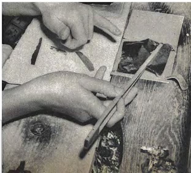
Above—Gold leaf, placed between sheets of goldbeater's skin, is hand-hammered for 8 hours until it is about 1/282,000 of an inch in thickness, as shown at right.
